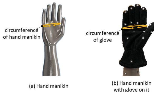
Fig. 1. Measurement location of circumference of (a) hand manikin and (b) hand manikin with glove.
