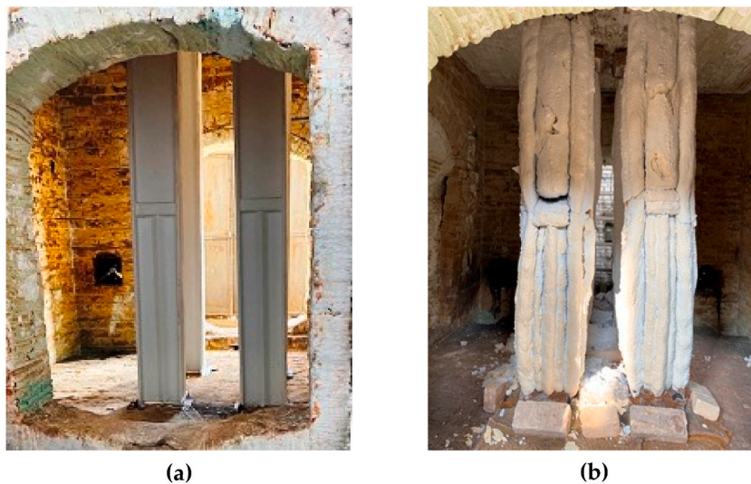
Fig. 6. Fire test of intumescent coating according to DSTU B V.1.1-14:2007 (EN 1365-4:1999 analog): a) steel columns before test; b) steel columns after 120 min exposure to fire.
