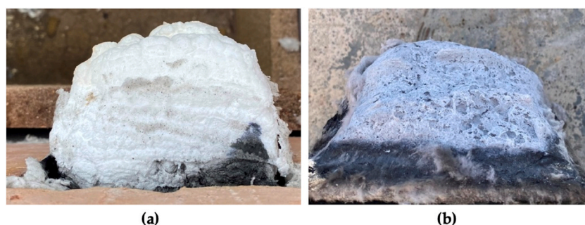
Fig. 17. Intumescent char obtained for intumescent composition similar to IC2 (Table 3) during fire test in laboratory-scale furnace: a – MC fiber content at 2.8 %, expansion factor K_1 = 34 , fire resistance R_1 = 52 min; b – MC fiber content at 5.2 %, expansion factor K_1 = 14 , fire resistance R_1 = 36 min. Dry coating thickness 1.8 mm for both, a and b.
