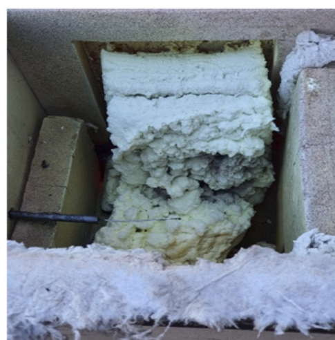
Fig. 5. Laboratory-scale furnace test at cellulose time-temperature curve: a) test setup; b) laboratory furnace; c) intumescent char after 120 min of fire test.
