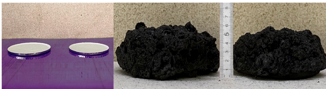
Fig. 3. Visualization of the experiment to measure volumetric intumescence factor.
