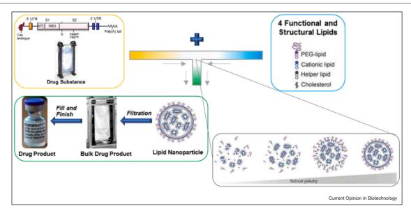
The mRNA drug-product platform process: mixing of the aqueous stream with the organic stream via a proprietary T-mixing process at fixed ratios and flow rates through a set flow path, provides self-assembly of the LNP formulation with the mRNA into nm-sized particles [36].
