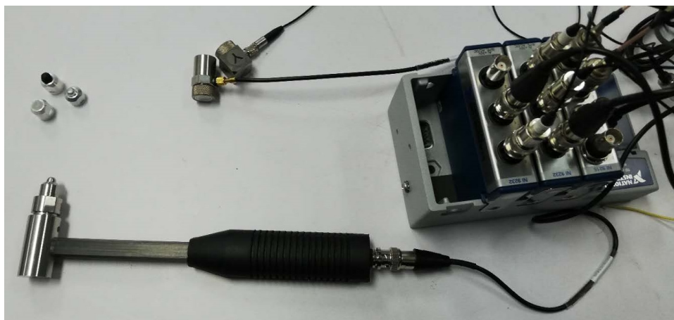
Figure 9. Data acquisition module for collision experiment.
