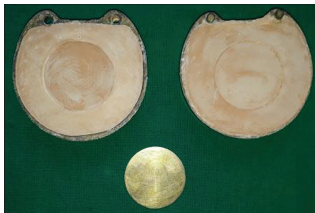
Figure 2: Mold space created with the help of metal die
