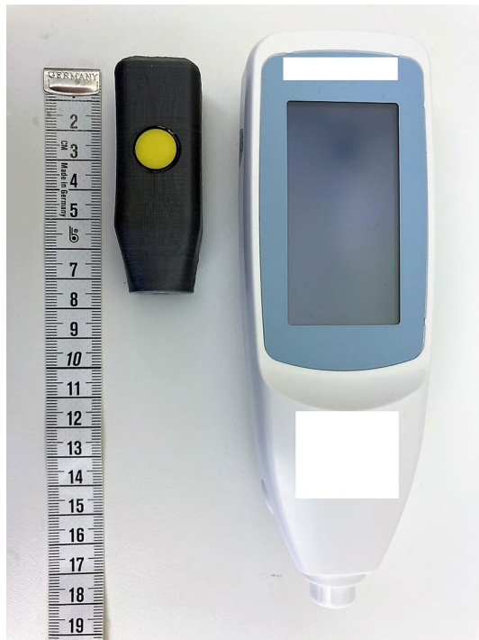
Figure 1. Photograph showing the two devices used in the study (JAISY to the left and JM105 to the right, measuring tape graded in centimeters).
