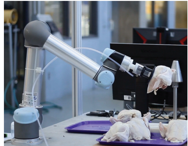
Figure 4. Demonstration of a human-guided grasp of a chicken front half by a robotic device.
