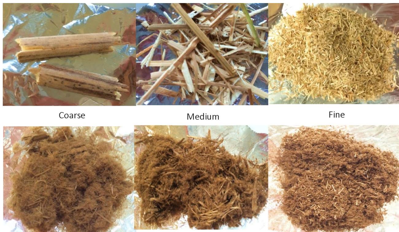
Figure 4. Photographs of (above) untreated biomass and (below) recovered pulps after pretreatment of Miscanthus with [TEA][HSO 4 ] at 120 °C for 6 h at bench scale using a biomass loading of 20 wt%.
