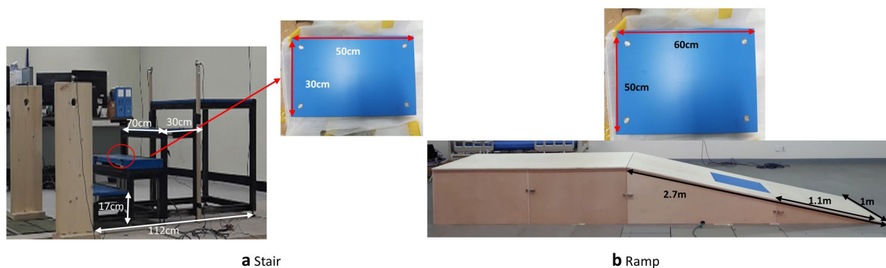
Figure 5. Instrumented (a) stairs and (b) ramp.
