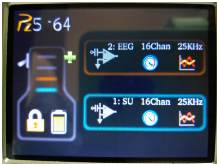
Figure 5: The GUI on the pre-amplifier. It allows EEG recording parameters (e.g., sampling frequency and referencing preference) to be set. Please click here to view a larger version of this figure.
