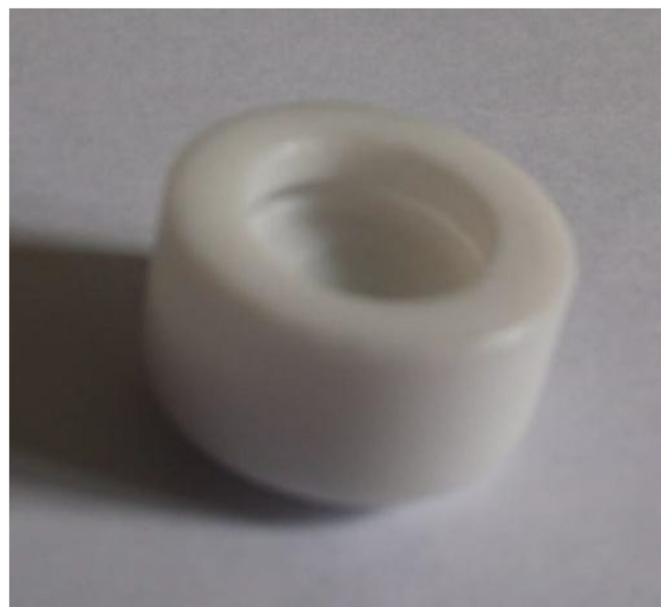
Figure 2. Rotating disk sorbent extraction (RDSE).
