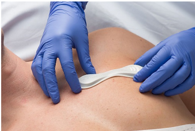
Fig. 1. The VitalPatch®, a single-lead, wet-electrode device that collects electrocardiogram and triaxial accelerometry data, used for the AccelerateIQ™ platform.
