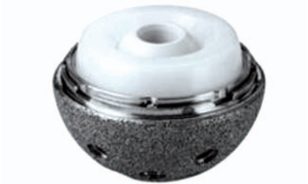
Fig. 1. A dual mobility acetabular hip implant has a bigger hemispherical polyethylene (PE) liner than an acetabular cup, causing its PE liner opening to be smaller than the diameter of a femoral head.
