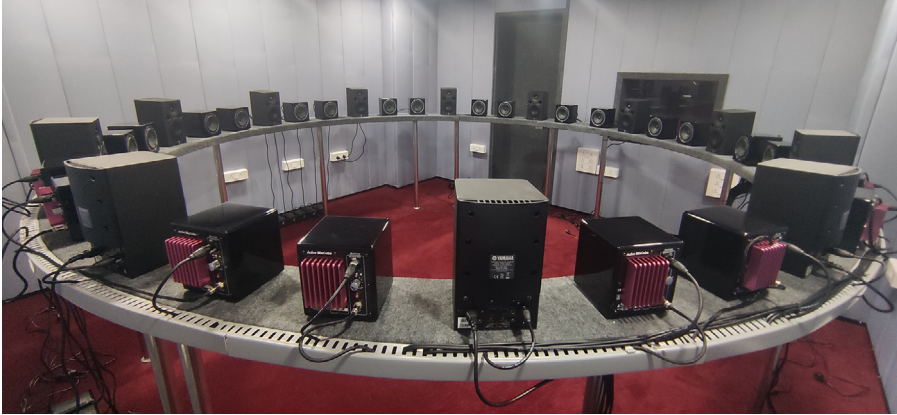
Fig. 4. Thirty-six loudspeakers positioned on a circular stand installed in the laboratory.
