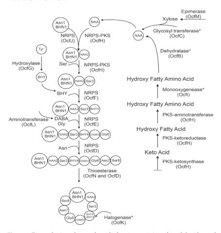
**Figure 2.** Biosynthetic pathway of occidiofungin consisting of a polyketide synthase pathway and non-ribosomally synthesized peptide synthase pathway. Steps which are uncertain in when they occur are marked with an asterisk. Adapted from Gu et al [12].
