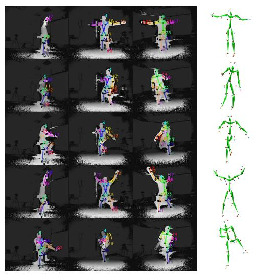
**Figure 15.** Five samples of the method results are illustrated in rows. At the left side of the figure, the multi-view input along with the FCN reflector-set estimates are presented, while, at the right side, their corresponding 3D optical and motion capture outcomes are shown.
