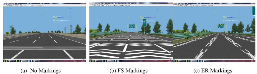
Fig 3. Experimental scenarios for deceleration markings used in the study. (a)No markings. (b) FS markings. (c) ER markings.
