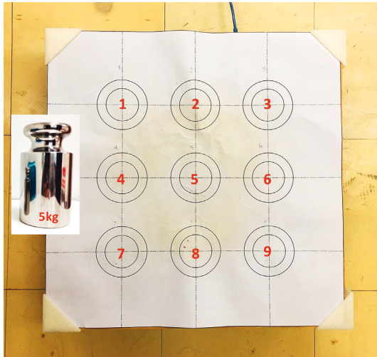
FIGURE 3: Nine positions and a 5 kg weight for testing SBAP accuracy.
