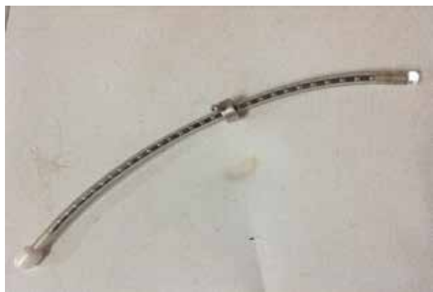
Fig. 1. Re-usable rectal marker for localizing rectum during applicator placement
