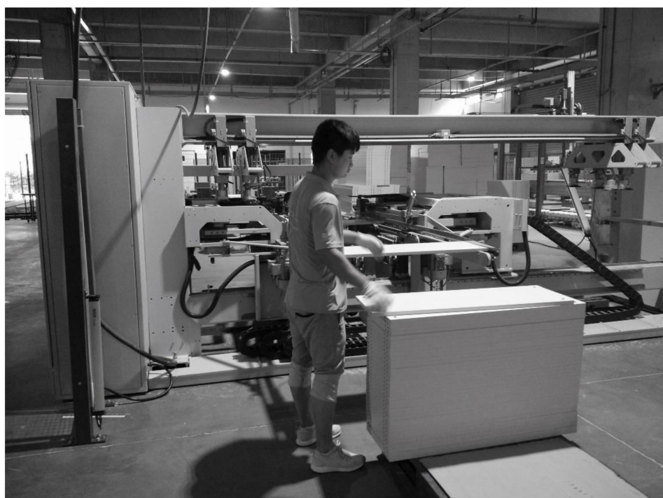
Figure 1. Handling panel boards to the inlet of six-row drilling machine (photo from a furniture manufacturing factory in China).
