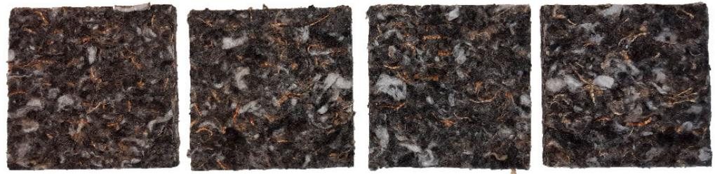
Figure 4. Samples for measurement of thermophysical properties by EDPS method.
