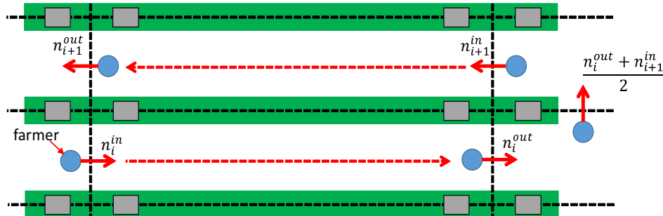
Figure 4. Passage restriction. A farm laborer can move from one passage to the next only by walking to the end of a passage. Thus, the farm laborer must be in the same passage from n_i^{in} to n_i^{out} .
