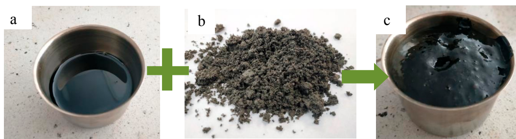
Figure 3. (a) 20 grams of 20/30 asphalt in a temperature of 135 °C; (b) Na-P1 zeolite soaked with water; (c) foaming effect of asphalt caused by water releasing from the zeolite.
