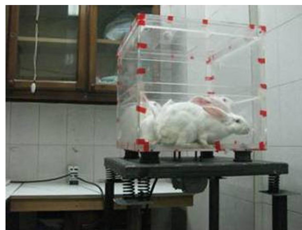
Figure 1. Cross-sectional View of Transparent Poly Carbonate Plexiglas Vibration Chamber Assembled on a Vibrating Platform Consisted of a Three-Phase Body Vibrator (Model ITAL VIBREH; M3/65; Italia) for Creating Vibration and an Inverter (Model LG; 0.37 KW IG5A-4; Korea).
