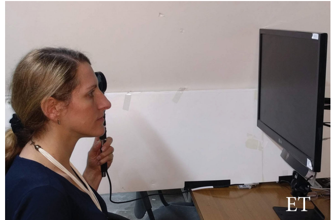
Figure 1. Experimental setup for eye tracking part of experiment. Participants sat at a distance of 40 cm from the monitor. The IR filter was placed in front of the eye by the examiner and was synchronized with the eye tracker, attached to a free-standing carrier at a distance of 60 cm (ET).
