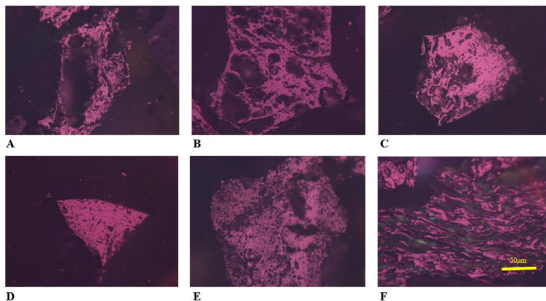
**Figure 3.** Images of semi-coke. (A) Larger cavity, vitrinite-derived; (B) network, vitrinite-derived; (C) fused and unfused particles; (D) unfused solid particle; (E) massive particle with more porosity; and (F) unfused particle with partially original structure. Optical microscope photos under crossed polars, oil immersion, and a  $1\lambda$  retarder plate.
