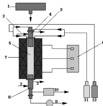
(1) Power feeder. (2) Cooling water inlet (3) Cooling water outlet (4) Combustion reactor
