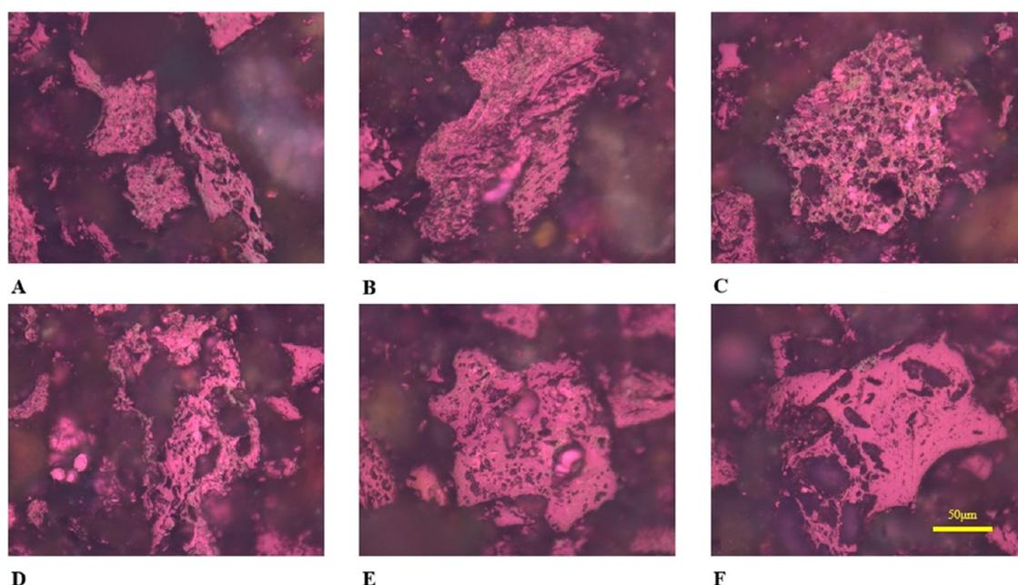
**Figure 6.** Images of unburned chars from coke breeze. (A, B) Anisotropic, mixed dense; (C, D) anisotropic, vitrinite-derived; (E) anisotropic, mixed porous; and (F) isotropic, with little anisotropic, inertinite-derived. Optical microscope photos under crossed polars, oil immersion, and a  $1\lambda$  retarder plate.
