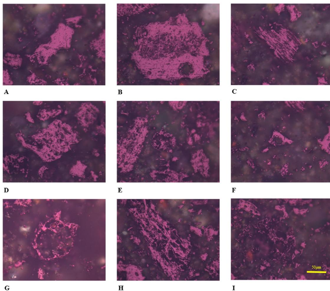
**Figure 5.** Images of unburned chars from semi-coke. (A) Solid; (B) inertoid; (C) fusinoid; (D) mixed dense; (E) mixed porous; (F) crassispheres; (G) tenuispheres; (H) crassinetwork; and (I) tenuinetwork. Optical microscope photos under crossed polars, oil immersion, and a  $1\lambda$  retarder plate.
