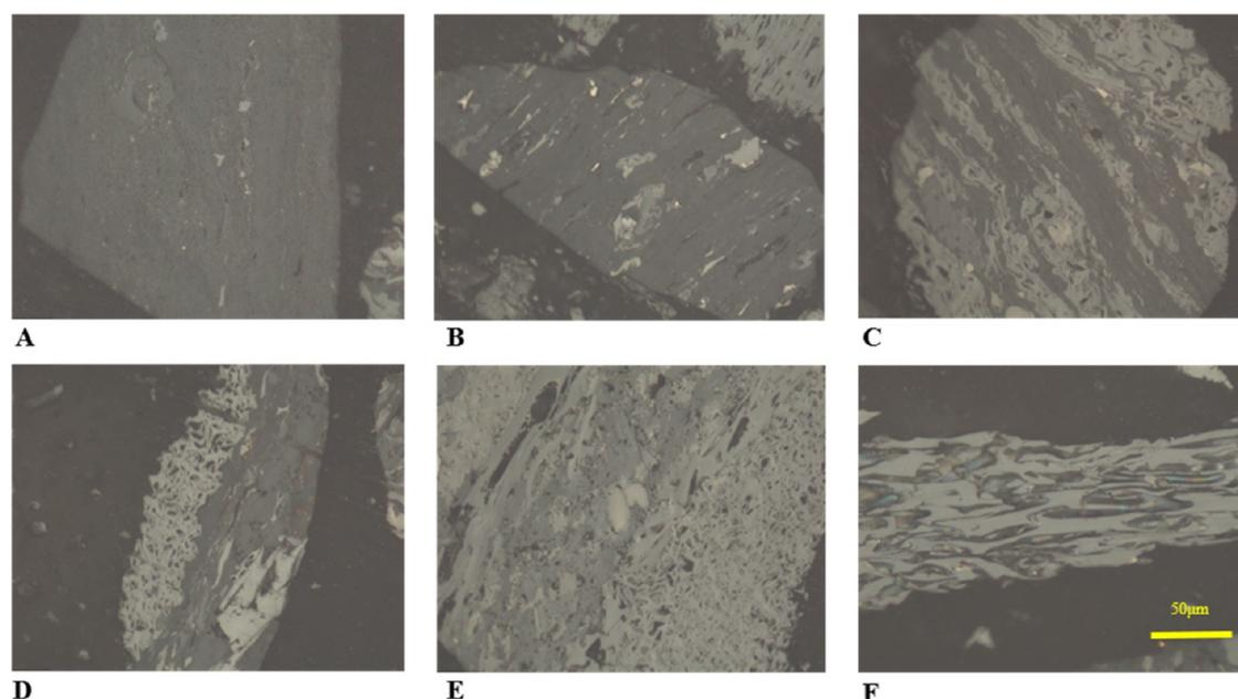
**Figure 2.** Images of low-rank non-caking coal: (A, B) vitrinite; (C, D) vitrinite and fusinite; (E) fusinite and semifusinite; and (F) fusinite. Optical microscope photos were obtained under reflected light and oil immersion.
