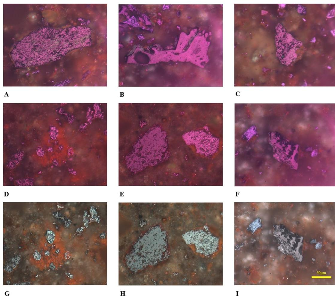
**Figure 7.** Images of fly ash from iron ore sintering. (A–C) Anisotropy; (D, E) isotropy; and (F) the intermediate particle is anisotropy, whereas the left is isotropy. (A–F) Optical microscope photos under crossed polars, oil immersion, and a  $1\lambda$  retarder plate. (G–I) Optical microscope photos under reflected light and oil immersion.
