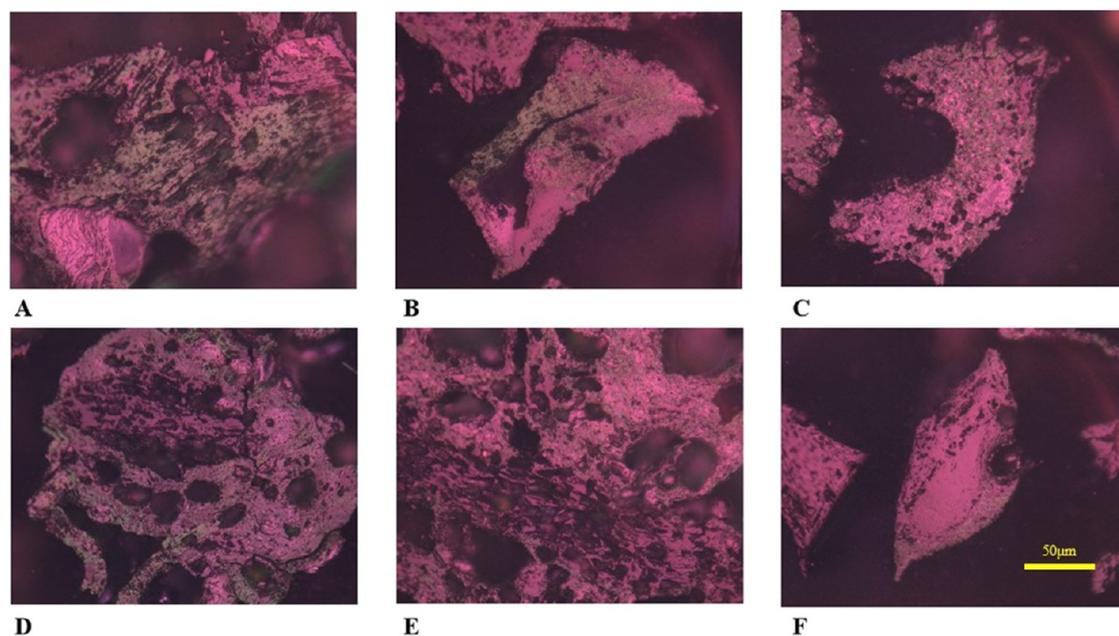
**Figure 4.** Images of coke breeze. (A–C) Anisotropic and (D–F) anisotropic, with included isotropic images. Optical microscope photos under crossed polars, oil immersion, and a  $1\lambda$  retarder plate.
