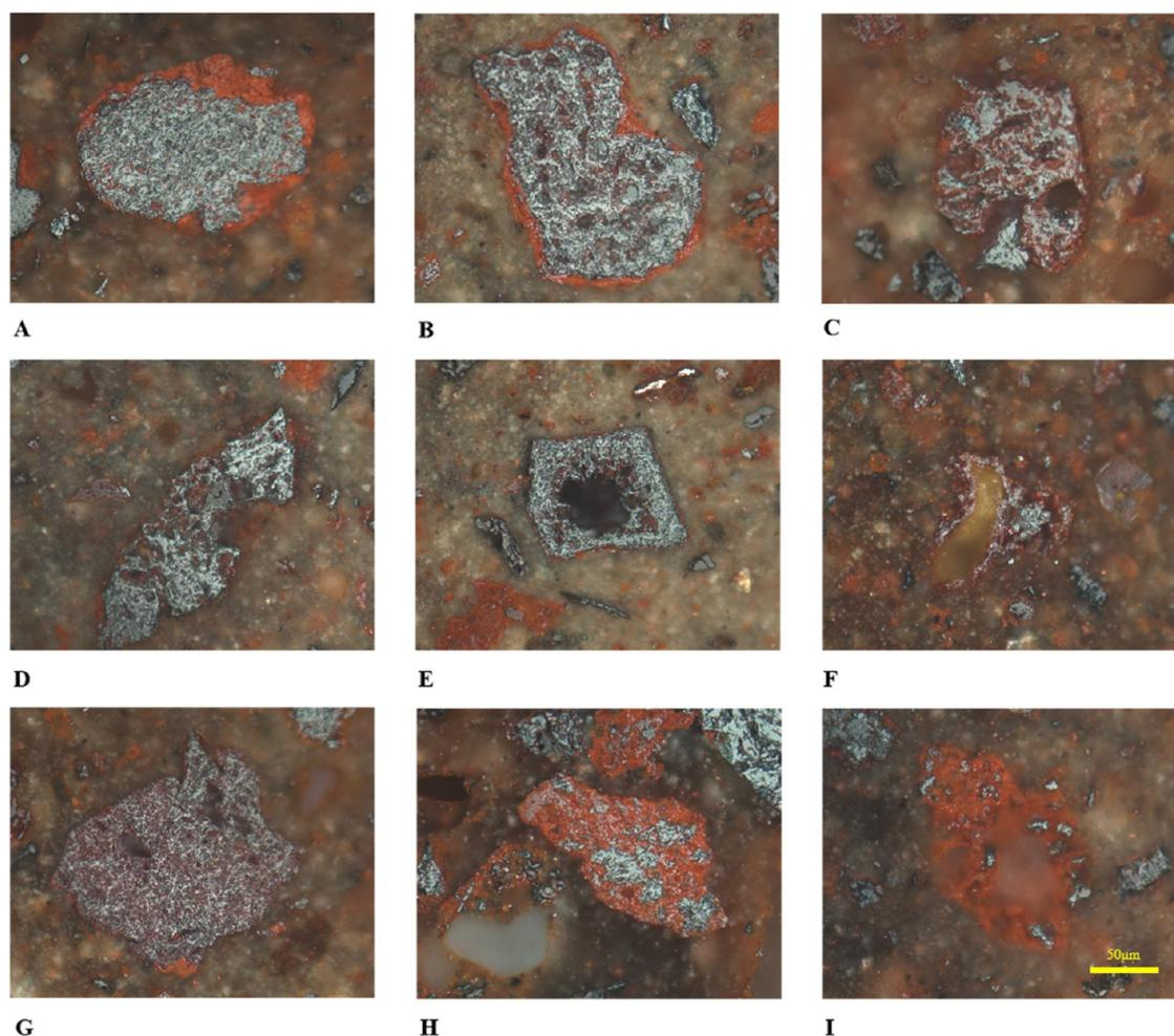
**Figure 8.** Images of unburned char derived from semi-coke of the iron ore sintering. (A) Dense particle; (B) dense particle with more porosity; (C) mixed dense; (D) crassisphere; (E) crassisphere; (F) tenuisphere; and (G–I) the unburned char and sinter. Optical microscope photos under reflected light and oil immersion, and  $\times 500$ .
