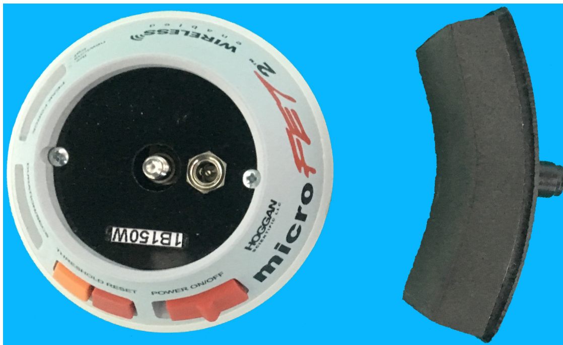
Fig. 7. Digital hand-held dynamometer MicroFet 2 (Hoggan Health Industries, Draper, UT).
