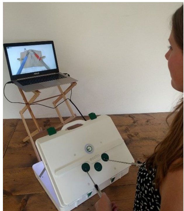
Fig. 1 Setup of the eoSim laparoscopic simulator
