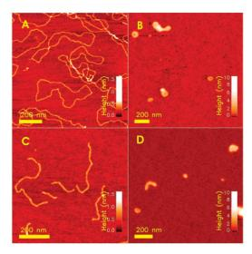
**Figure 6.** Tapping mode AFM height topographs of: uncomplexed pBR322 (**A**); and linear DNA (**C**); alongside with complexes of these formed when mixed with the chitosan C (0.01,162) (**B**, **D**) cDNA 4  $\mu$ g/mL and N/P = 1. Reprinted with permission from Danielsen et al. (2004) Biomacromolecules 5, 928–936 [120]. Copyright 2004 American Chemical Society.
