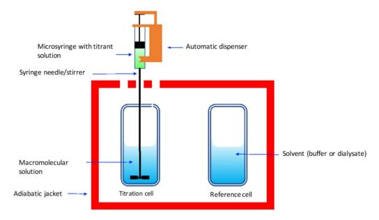
Figure 9. Schematic view of an isothermal titration calorimeter.
