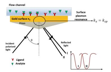
**Figure 7.** General principle of SPR, where n2 is the refractive index of medium with lower refractive index, E is the evanescent field amplitude,  $k_{sp}$  is the wavevector of surface plasmons, and  $k_x$  is the wavevector of photon.
