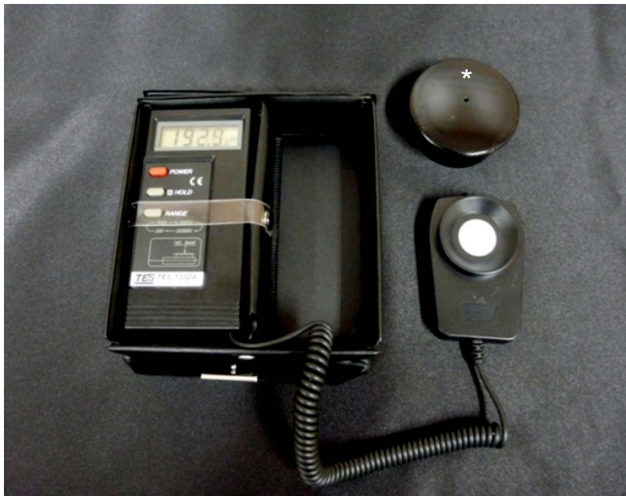
Figure 1. The TES Digital Light Meter and the model eye (asterisk) that can completely covered the photo sensor of light meter.
