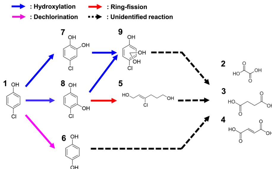
Figure 5. 4-CP oxidation, hydroxylation, dechlorination, and aromatic ring fission via neutral reactive species irradiation.
