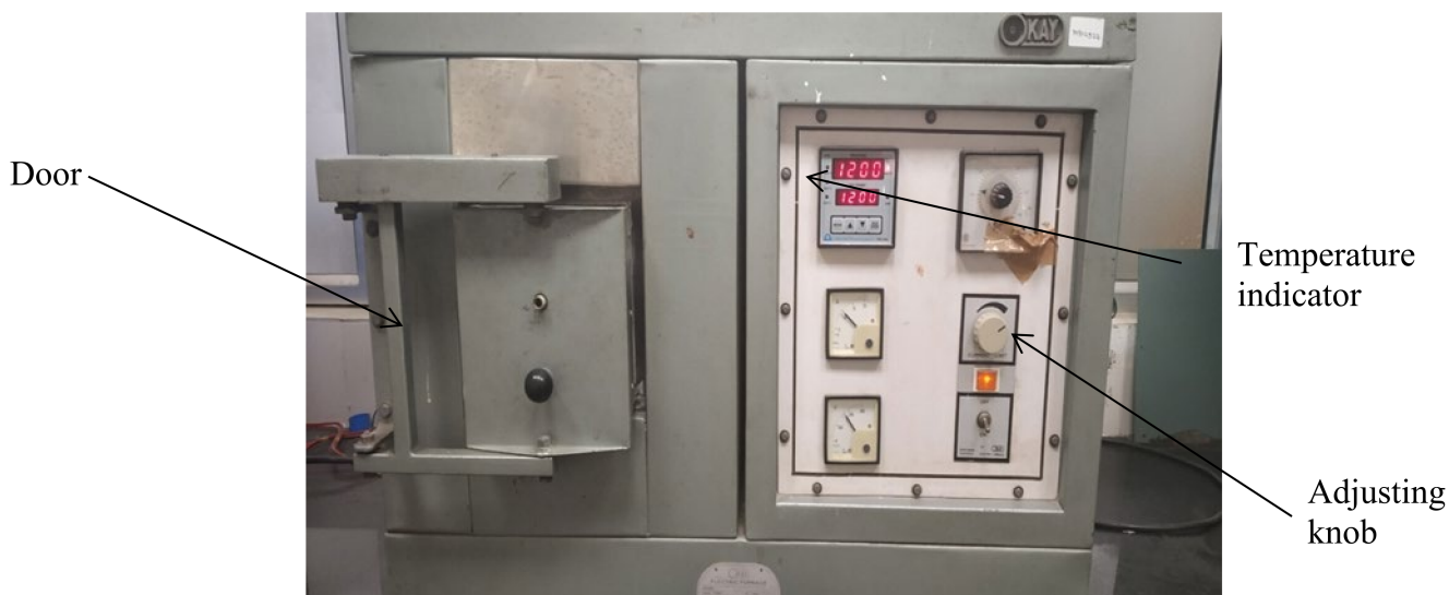
Figure 6. Electrical resistance based conventional heating setup.
