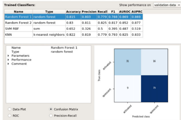
Fig. 3. The right half of the ml4bio software interface. The top shows a summary of all classifiers created during model selection, and the bottom shows detailed information on the performance of the selected classifier. Note that multiple classifiers can only be viewed during model selection. The user must select a single model and can no longer see the performance of other models once the test set is examined
