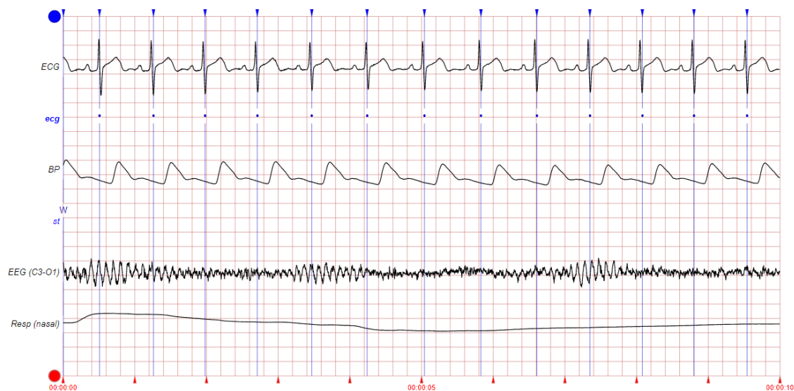
Figure 2. Examples of signals of interest for heartbeat detection: Blue vertical lines show the heartbeat annotations. This figure corresponds to slp04 record from MIT-BIH Polysomnographic Database.
