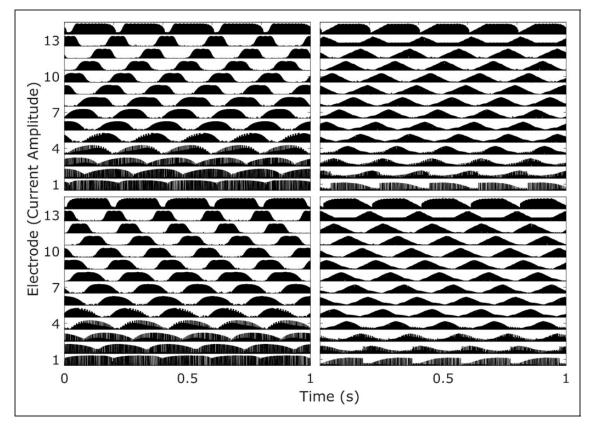
**Figure 4.** Electrodogram Plots of Density = 5 STRIPES Stimuli When Processed Using AB24's HiRes (Left Panel) and Optima (Right Panel) Programs. The top row shows UP STRIPES, and the bottom row shows DOWN STRIPES.
