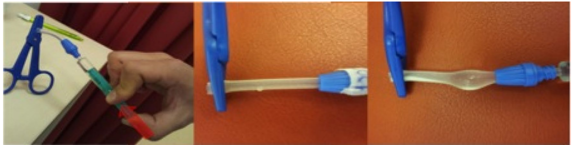
Figure 3. Intraluminal pressure exposure (left) to identify leakages such as e.g. liquid outlets (middle) and/or bulging (right).
