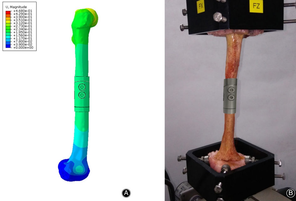
Fig. 4 FEA validation. To simulate the mechanical test as far as possible, the same boundary condition was set up for FEA. (A) Mechanical test. (B) FEA.
