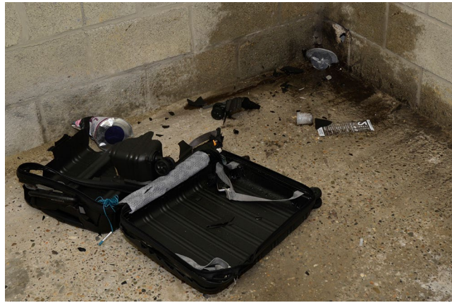
Figure 1. Post-neutralisation experimental setup. To disarm the IEDs, an RE70 M3 Plus Waterjet Disruptor was used, firing a ballistic water jet onto every IED. Variable destructive effects were observed throughout the five testings.
