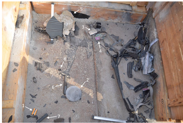
Figure 4. Post-blast experimental setup. Five IEDs were consecutively detonated with 7 g C-4. The arrows mark a few parts of recovered components: (1) battery, (2) lid of metal can, (3) mobile phone, (4) printed circuit board, (5) metal can, (6) handle and (7) combination lock of suitcase, (8) push button.
