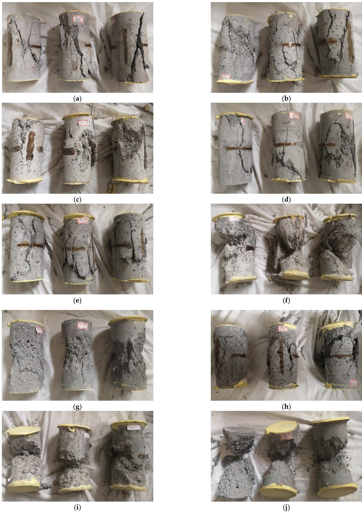
Figure 4. Failure modes of PFRGCs (a)F40-P0; (b) F40-P0.6; (c) F40-P1.2; (d) F60-P0; I F60-P0.6; (f) F60-P1.2; (g) F80-P0; (h) F80-P0.6; (i) F80-P1.2; (j) F100-P0.
