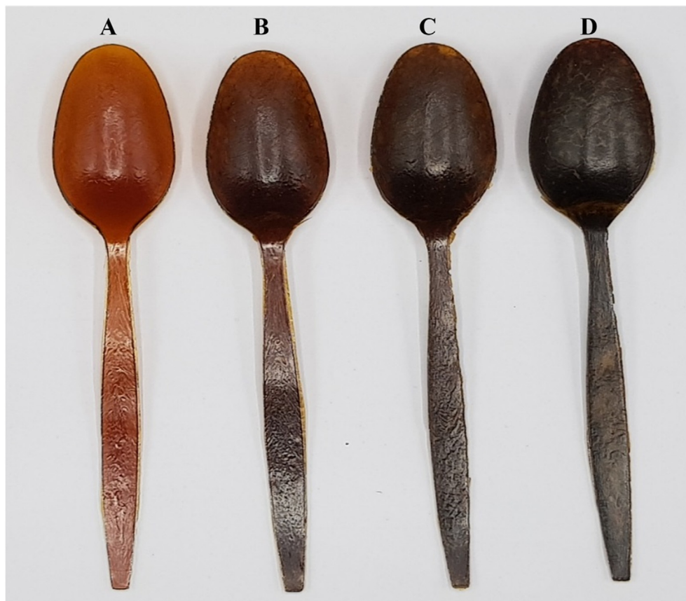
Figure 2. Digital photographs of SPI cutlery supplemented with different levels of morning glory stem fiber (MGSF), (A) SPI-CON, (B) SPI-MGSF-5, (C) SPI-MGSF-10, (D) SPI-MGSF-20. SPI-CON (SPI without MGSF), SPI-MGSF-5, SPI-MGSF-10 and SPI-MGSF-20 samples presented SPI without and with the addition of MGSF at different levels of 5, 10, and 20%, respectively.
