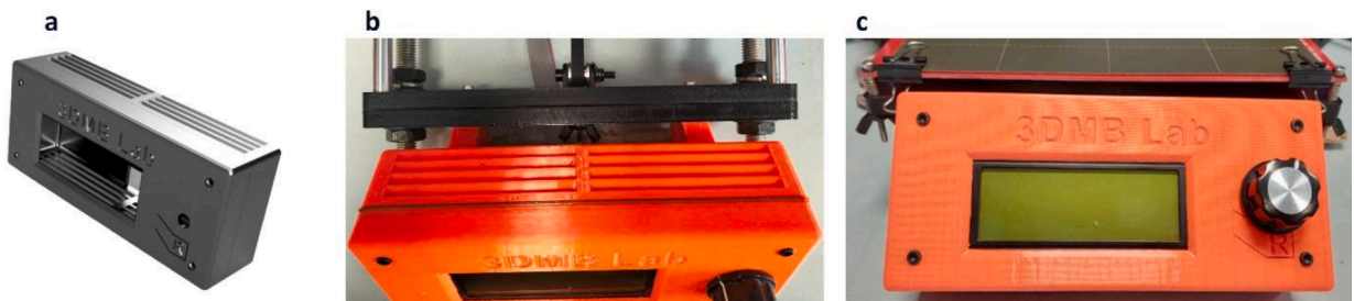
Fig. 11. Relocating the LCD by introducing the display box to new spot: (a) Render imaging of the new display box. (b) Top view of the installed LCD to the 3D bioprinter. (c) Front view of the LCD, attached to the acrylic body.
