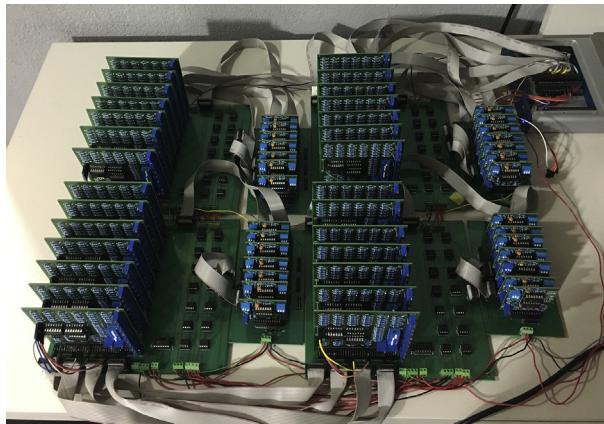
Fig. 6. Photograph of the experimental array using 28 nonlinear oscillators and their corresponding electronic couplers. The voltage of each oscillator was acquired by a DAQ card (NI USB 6363), shown at the top right corner of the photograph.
