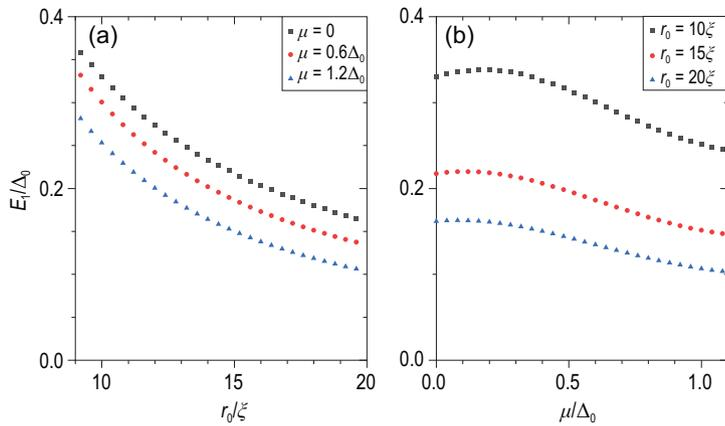
**Figure 4.** The scatter graphs of the first excited energy  $E_1$  of the Hamiltonian in Equation (11) with respect to (a) the superconducting nanowire's radius  $r_0$  for different chemical potentials and (b) the chemical potential  $\mu$  for different radii of nanowires with  $V_z = 4\Delta_0$ . Other parameters are the same as those in Fig. 3.
