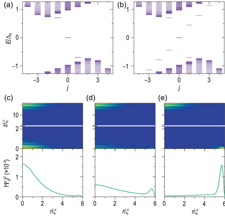
**Figure 3.** The spectra of the iron-based superconducting nanowire system in Equation (11) with the bottom layer effective ZF (a)  $V_z = 0$  and (b)  $V_z = 4\Delta_0$  at  $\mu = 1.2\Delta_0$ . (c)–(e) The MZM distribution  $|\Psi_0|^2$  near the top and bottom surfaces corresponding to  $V_z = 0, 2$  and  $4(\Delta_0)$  in sequence. The lower panels show the probability density  $|\Psi_0(j)|^2$  on the bottom surface. Other parameters are the same as those in Fig. 1.
