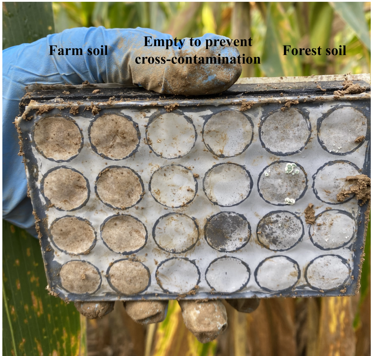
Supplementary Figure 1: A constructed microbial trap with an 18 \mu\text{m} nylon membrane. Microbial trap had been deployed into an agricultural corn field.
