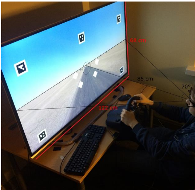
Figure 1. The experimental set-up. During the experiment, the display was the only light source.
