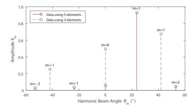
**Figure 4.** Power spectrum produced by a five-element array receiving a signal from a source at an angle of 25°. When the samples from the outer elements are removed, then the array produces a new spectrum with different characteristics (shown as the dotted lines in the figure).
