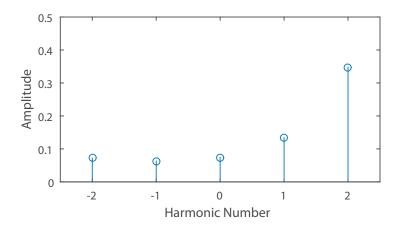
**Figure 3.** Power spectrum produced by a single sinusoidal source when sampled by a uniformly switched five-element time modulated linear array. The signal is impinging on the array at an angle of 45°.
