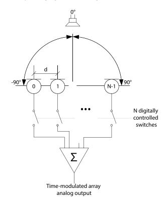
Figure 1. Typical schematic of an N element time-modulated array with d spacing.
