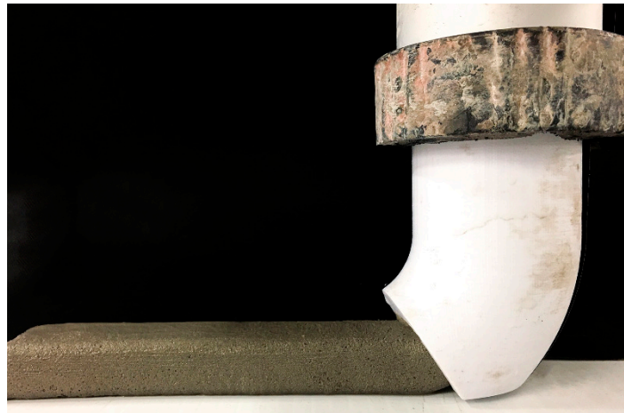
Figure 2. The geopolymer mortar being extruded from the nozzle.
