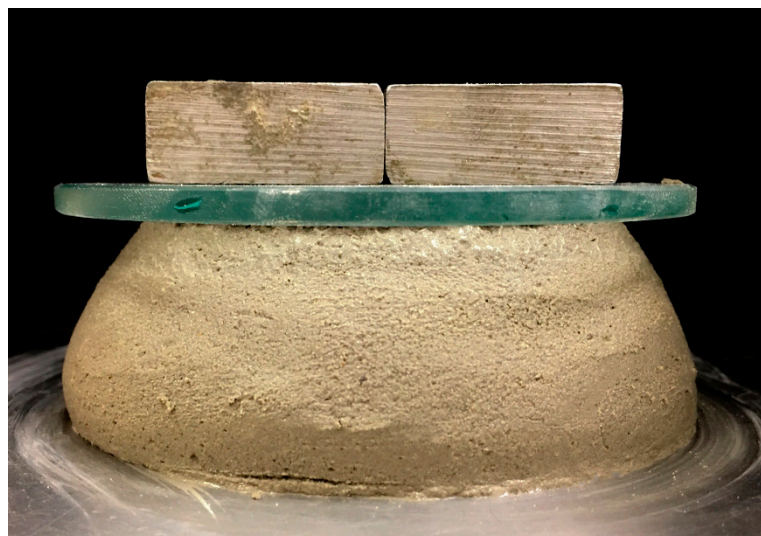
Figure 3. The shape-retention ability test setup.
