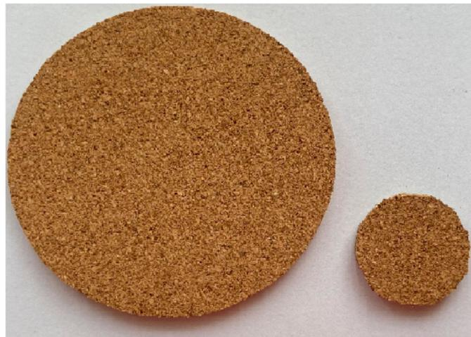
**Figure 2.** Foxtail millet husk powder composite sample for measuring sound absorption.
