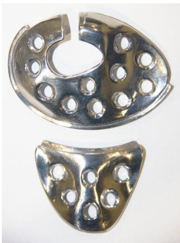
Fig. 3 A prototype of the implant manufactured by CNC machining. (Upper part is the femoral component of the implant, and lower one is the tibial component)
