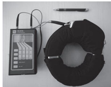
FIGURE 2: The induction clamp-on meter of limb current (HI-3702 probe and HI-4416 monitor).
